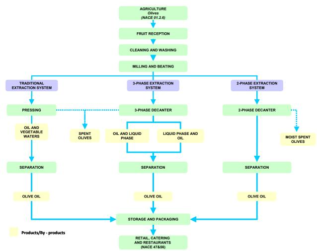
Figure 5.1: Main stages of olive oil production.
