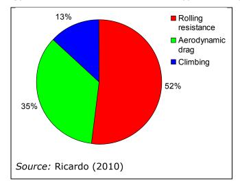
Figure 3.20: Energy demand from a 44 t HGV over a typical driving cycle in the UK
