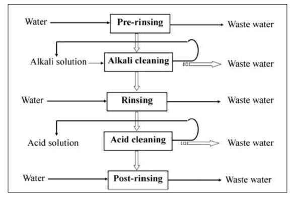
**Figure 3.7:** Conventional cleaning steps in the CIP process in the dairy industry
