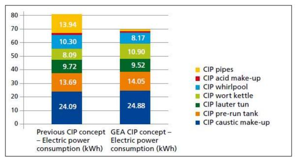
**Figure 3.9:** Electric power consumption per CIP process at the Gutmann brewery, Titting, Germany
