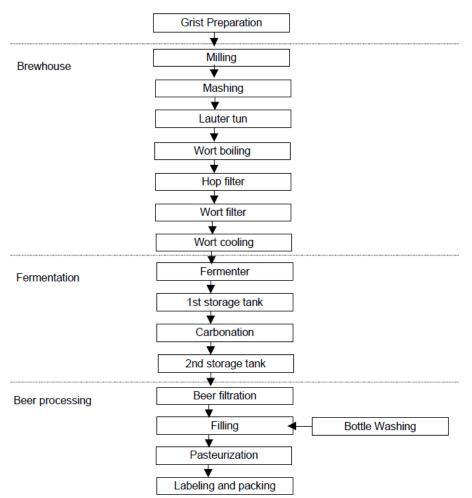
Figure 7.8: Overview of the main processes of the beer manufacturing (Galitsky et al., 2003)
