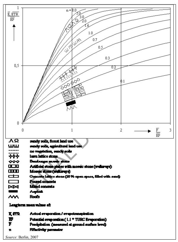
Figure 2.4: Representation of the Bagrov Equation for selected values of n (effectivity parameter) for different land uses or soil types
