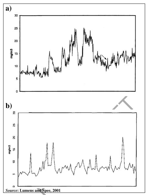
Figure 5.34: Dust concentration in a closed room. Recess milling (a) and sawing (b)
