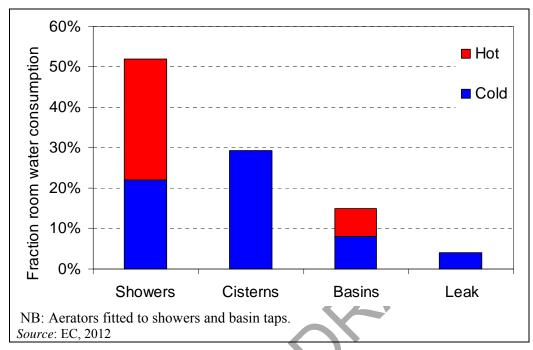
Figure 6.2: Breakdown of water consumption across eight rooms in a hotel obtained from a study employing sub-metering of flow rates through pipes to individual fittings
