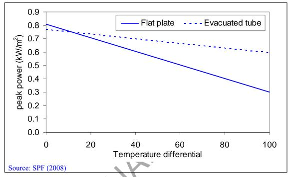
Figure 3.42: Variation in standard test peak power output from two solar collectors relative to temperature differential (maximum water temperature minus ambient temperature)
