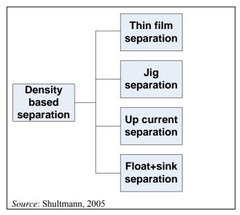
Figure 7.3: Water-based separation techniques
