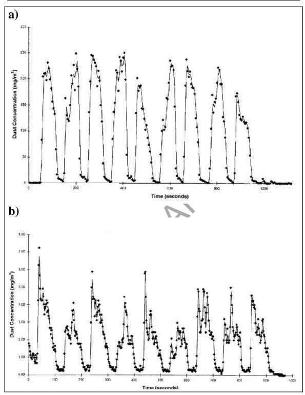
Figure 5.35: Dust concentration during cuts without water dust suppression and with water supplied using an electric pump to supply water at 0.5 L min<sup>-1</sup>
