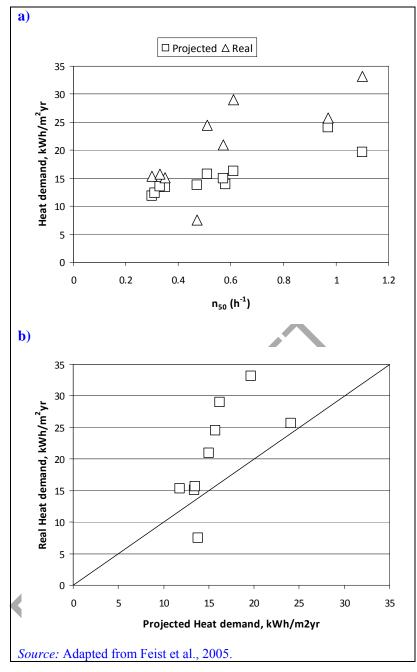
Figure 3.28: Heat demand vs. air leakage (a) and measured heat demand vs. projected heat demand
