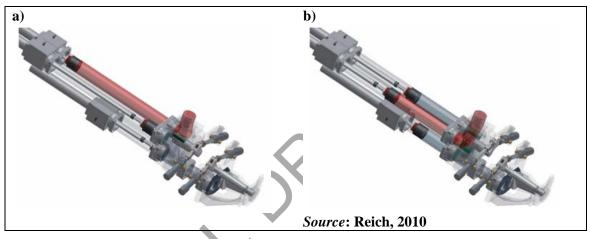
Figure 5.40: Pumping of concrete with continous flow: a) first cylinder laoding phase b) second cylinder loading phase
