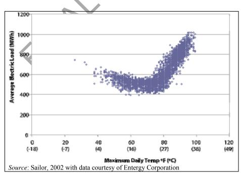
Figure 2.10: Electrical load of buildings in New Orleans vs. maximum daily temperature
