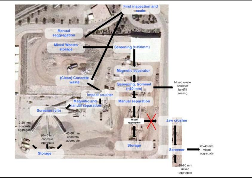
Figure 7.10: Overview of the recycling process at SalmedinaTri
