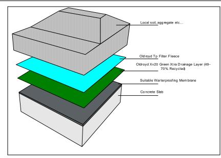
Figure 3.20: Typical layer build-up of brown roofs
