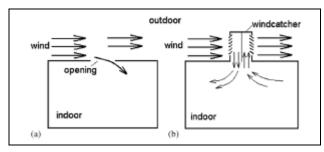
Figure 3.37: Windtower options: a) single opening, b) common windcatcher
