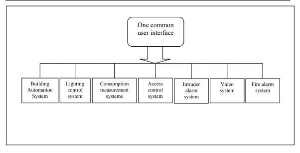
Figure 6.1: Integrated building management system
