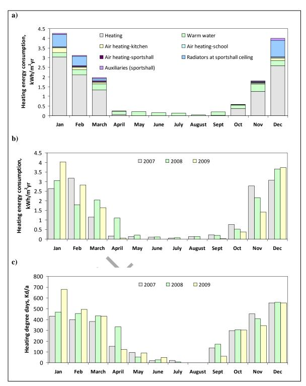
Figure 3.32: a) Monthly heating energy consumption at Riedberg school during 2009 for several internal processes. b) Monthly heating energy consumption (excl. hot water preparation) in 2997, 2008 and 2009. c) Monthly value of heating degree days in Frankfurt in 2007, 2008 and 2009.
