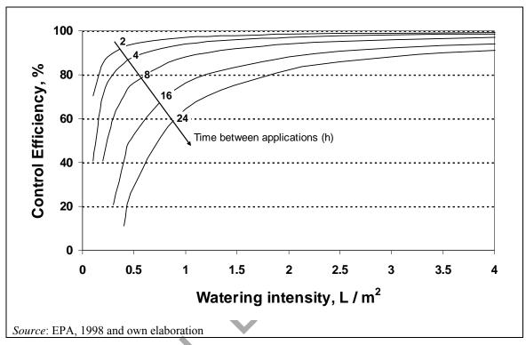
Figure 5.33: Dust control efficiency vs. watering intensity and time between applications
