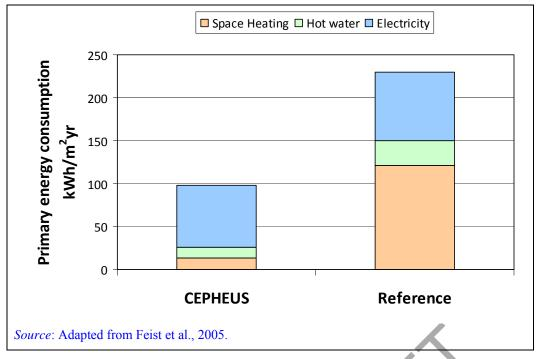
Figure 3.29: Comparison of primary energy consumption of all CEPHEUS projects with new buildings from 2005 according to building codes
