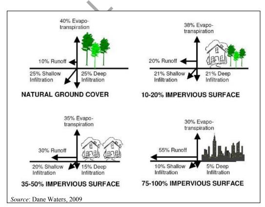
Figure 2.3: Impact of impervious area on hydrologic fluxes
