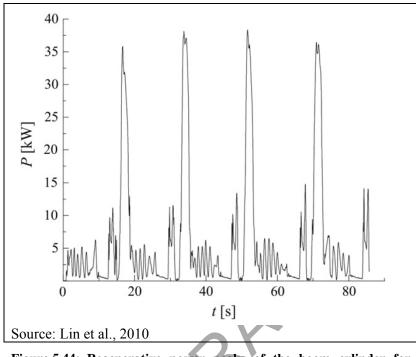
Figure 5.44: Regenerative power peaks of the boom cylinder for several consecutive digging works
