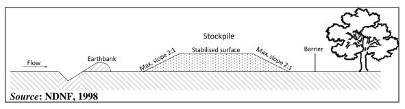
Figure 5.32: Pile configuration to avoid dust generation
