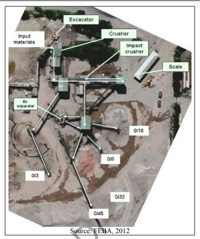
Figure 7.8: Aerial view of a recycling plant
