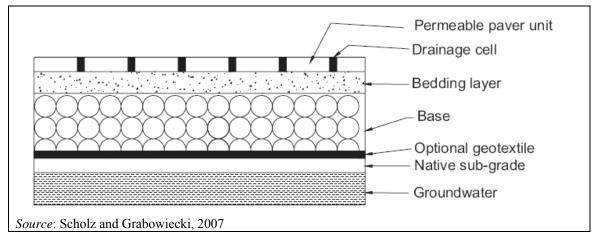
Figure 3.47: Typical schematic layout of a permeable pavement
