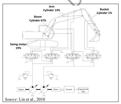
Figure 5.43: Structure of a hydraulic excavator and the regeneration potential of energy in an hybrid system
