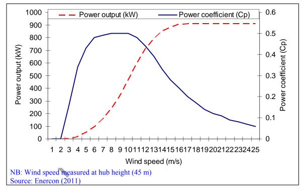
Figure 3.43: Evolution of power output and conversion efficiency (Cp) with wind speed for a 900 kW turbine
