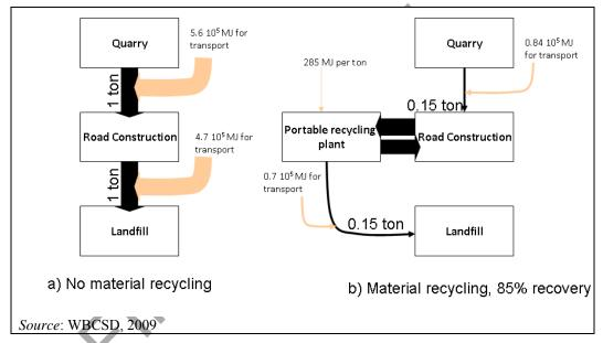
Figure 8.3: Energy and material flows without and with recycling for road construction
