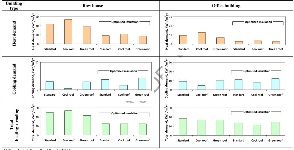
Table 3.21: Heat, cooling and total energy demand of a row house and an office building with different types of roofs
