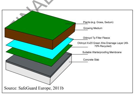
Figure 3.21: Typical layer build-up of flat green roofs
