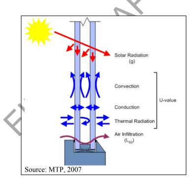
Figure 3.25: Energy flow through a window
