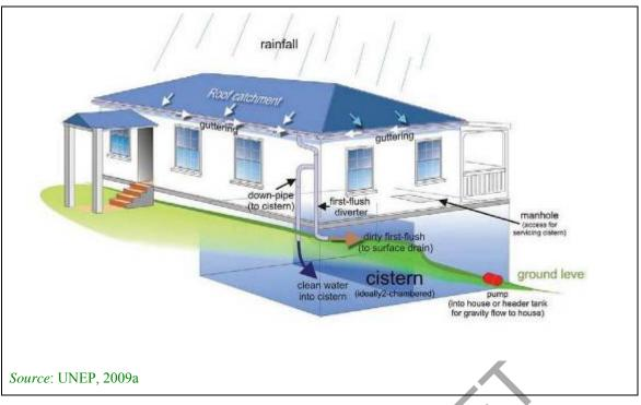
Figure 3.52: Example of a domestic underground Rainwater Harvesting system
