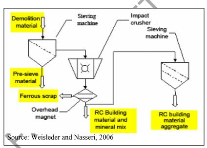
Figure 7.4: Example of a concrete recycling process
