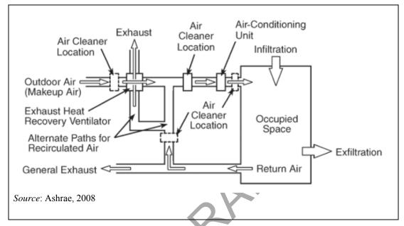
Figure 3.18: Design example of a ventilation system
