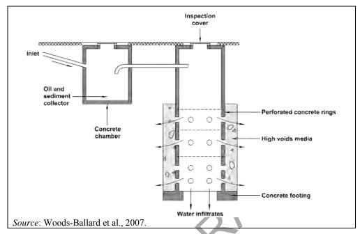
Figure 3.48: Soakaway with pretreatment device
