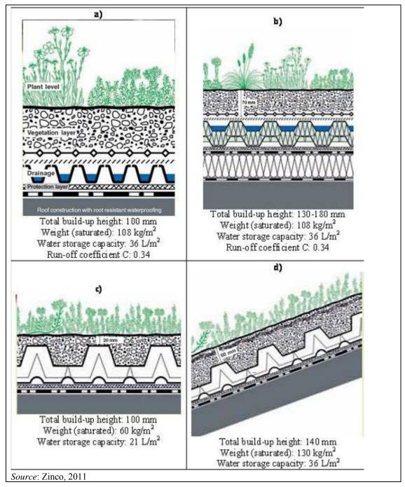
Figure 3.22: Green roof designs for: a) normal extensive, rock type plants, b) combined with thermal insulation, c) low weight option and d) pitched roof
