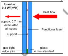
Figure 9.1: Structure of vacuum insulation glass<sup>45</sup>
