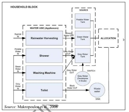
Figure 3.46: Components of a model in a household block (example)
