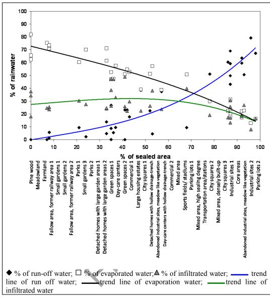
Figure 2.5: Run-off water performance in Berlin for different sealing degrees
