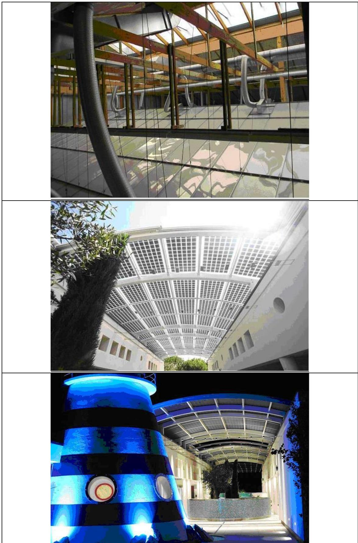
**Figure 9.16:** Window panels in the roof and suspended translucent ceiling allow natural light into the wash area of Kühlungsborn Campsite (above) and translucent retractable roof of the wash area in the Jesolo International Campsite (below)
