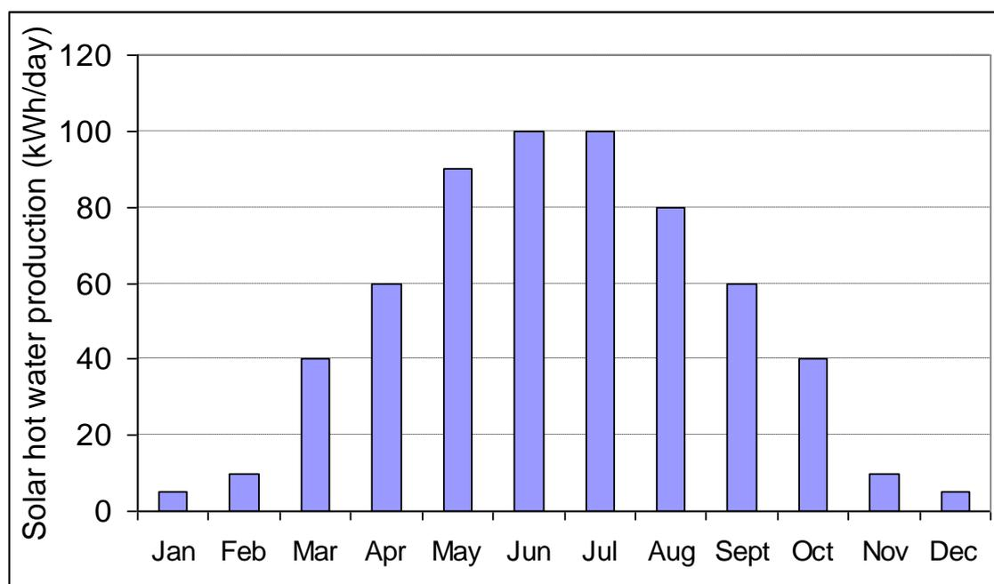
**Figure 9.17:** Maximum daily solar hot water production throughout the year for 41 m<sup>2</sup> of flat-plate solar panels installed on the east facing roof of a washroom in Seehof Campsite
